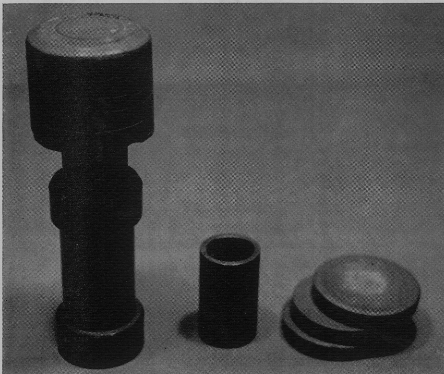
Figure 3. Loaded bomb with weight in place and auxiliary foot and weights
